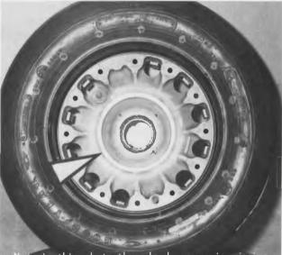
Note in this photo the wheel spacer is missing.
