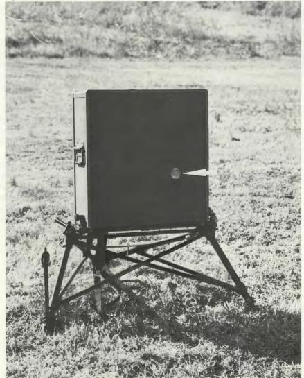
The complete TALAR transmitter weighs only 50 pounds making it highly transportable and requires only about five minutes to set up. Note the borescope sight used for establishing the glide path.
