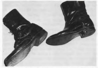
Note the lack of ankle support provided by the non-regulation boot. Check the split side seam near the sole.
