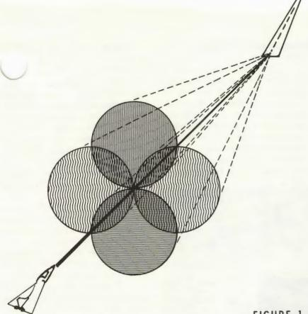
the glide slope and the localizer ourse (Figure 1). This differs cally from the conventional ILS oftem which employs two separate transmitters, one located at the far end of the runway which radiates localizer information, and the other positioned to one side of the runway for glide slope information. The TALAR transmitter is positioned on runway centerline near the runway threshold (approximately 300 feet prior to the runway and on the extended runway centerline).
