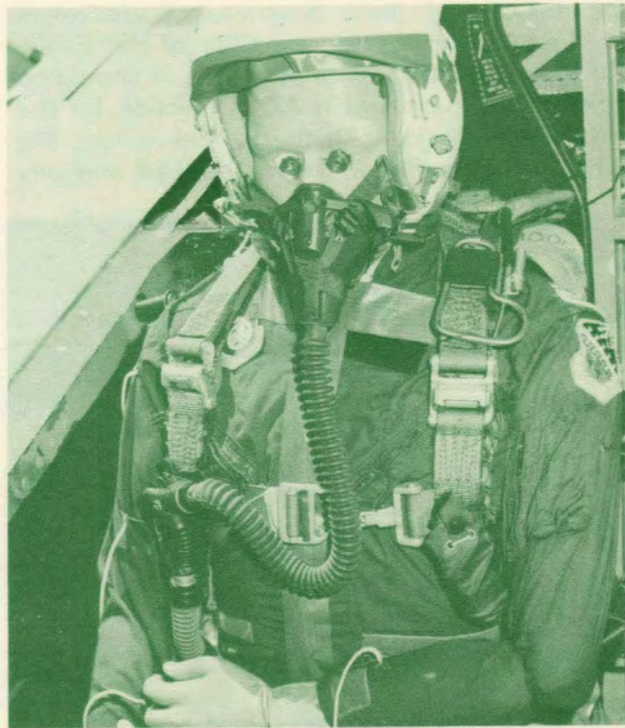
"Dummy" positioned in rear cockpit of TF-15 prior to first ground tests of canopy-off program. Helmet contained 15 sensors. An eye-mounted transducer was also used to measure impact pressures.
