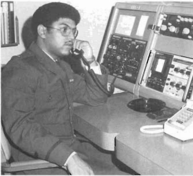
Using the voice communication capabilities of the AN/GRC-189 Ground Satellite Communications Terminal, an AFCS officer operates the radio control-head supporting the system.
