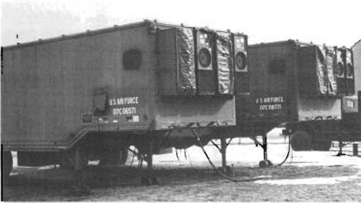
Mobile Digital Subscriber Terminal Equipment provides message service when system improvements or combat exercises preclude the use of fixed AUTODIN facilities.
