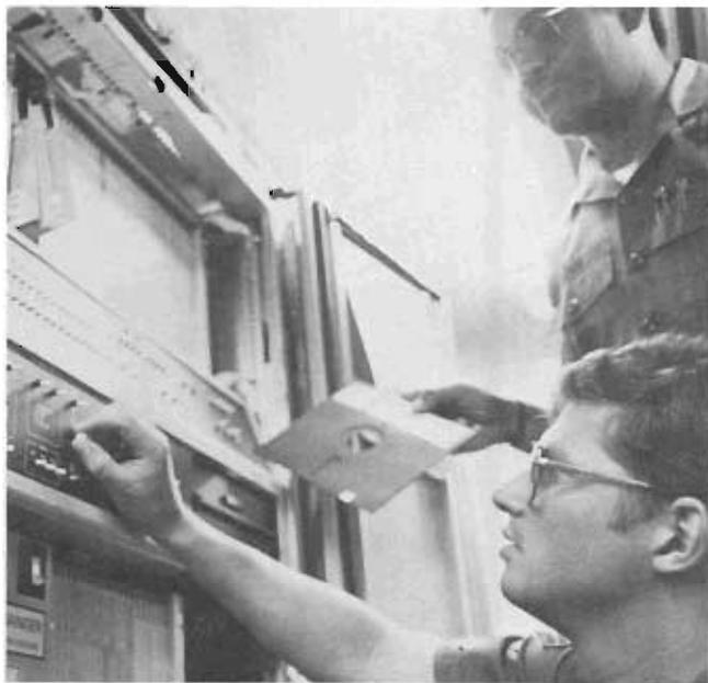
SrA Larry Psenick, 1956th Communications Group, Yokota AB, Japan, sets address switches on a disk controller while TSgt Charles Ross, 1982d Communications Squadron, Kunsan AB, Korea, stands by with a boot floppy disk. The two were testing part of the data processing Tactical Shelter System, a transportable base data processing system designed to provide automated base level information systems support under wartime or contingency operations.
