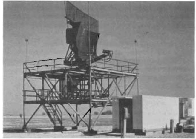
An AN/GPN-20 radar surveillance antenna with the fixed site/false target antenna mounted on top of the radar antenna.
