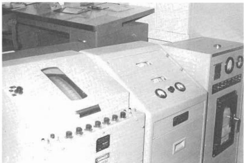
This portion of the AN/TMQ-11 indicates the temperature and humidity information it receives from the remote transmitter located on the airfield.
