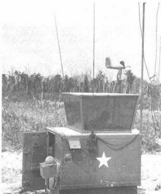
Portable air control towers such as this one were set up to direct planes into areas where permanent or fixed equipment did not exist.
