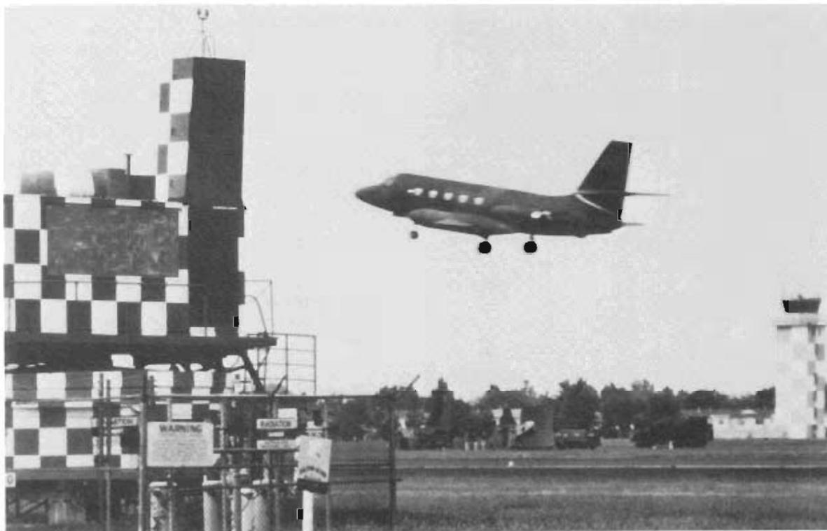
An AFCC C-140A aircraft makes a flight check of a final approach control radar. While logging more than 145,000 flying hours, AFCC's six specially equipped planes have had no major mishaps. In 1985 alone they flew 4,000 hours in support of their mission and played a major role in the Air Force flight safety record set in that year.
