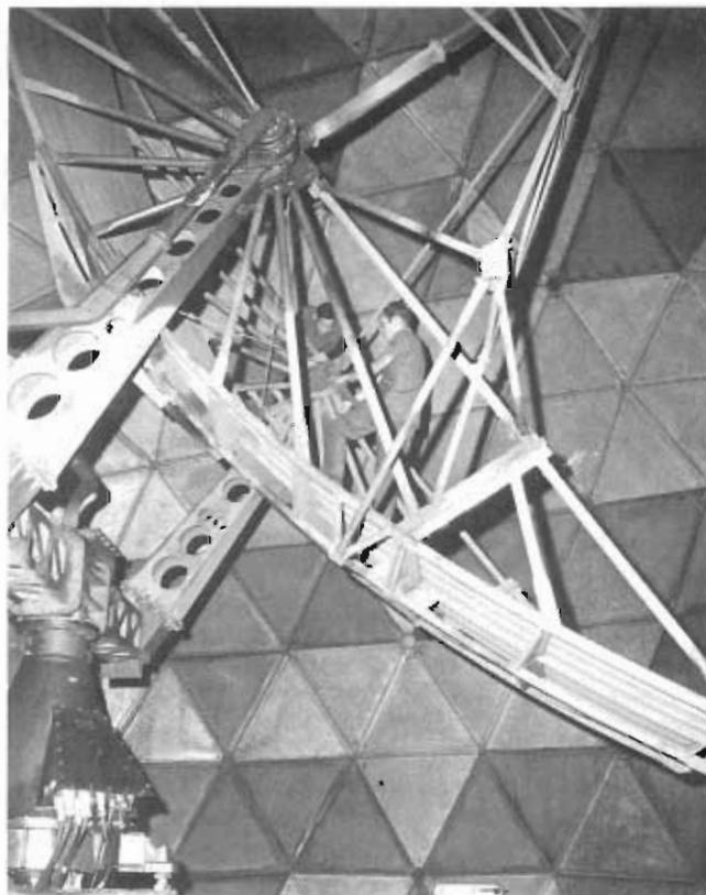
Maintenance personnel from the USAF and the Royal Thai Air Force work together to perform a periodic check of the slip ring on an AN/FPS-89 radar set at Udorn AB, Thailand.
