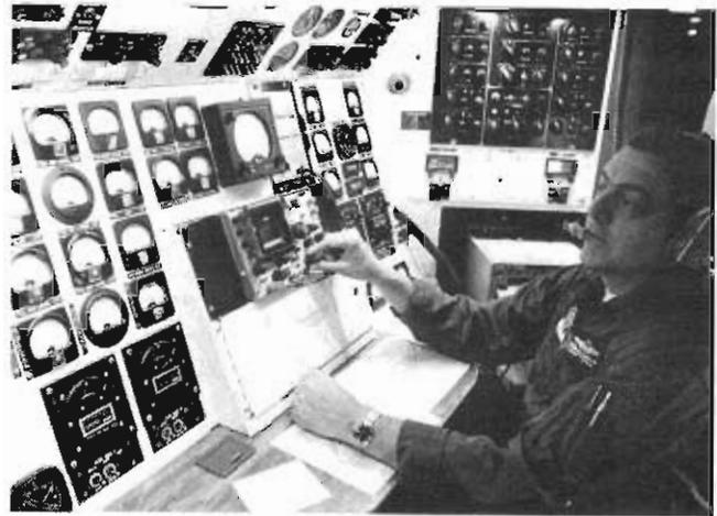
Flight checking equipment on board AFCC's C-140A aircraft.
