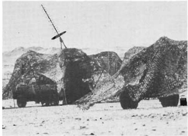
Camouflage netting helps conceal this mobile satellite terminal and helical antenna.
