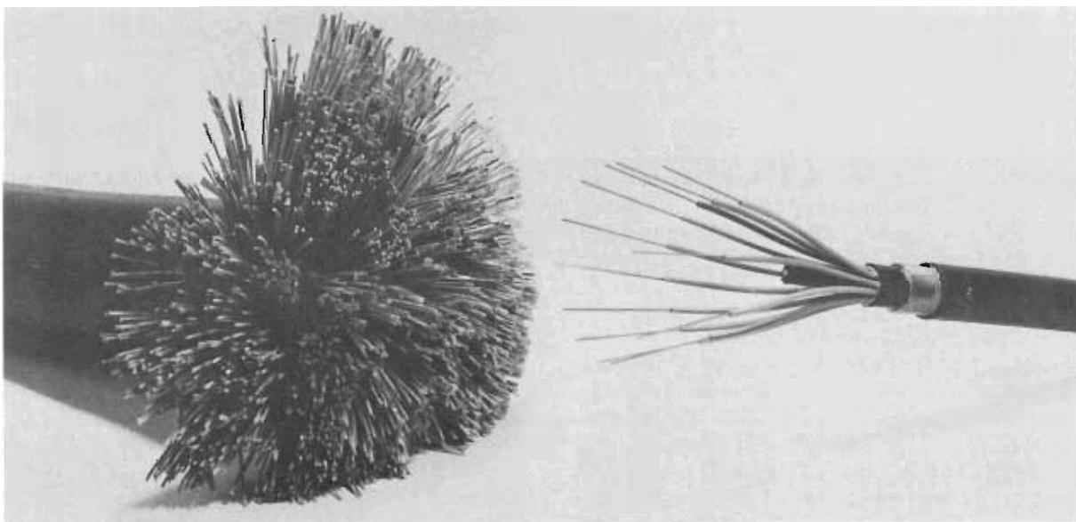
Existing communications wire, left, compared to replacement lightguide fiber optic cable. Fiber optic transmissions move along at a speed of 186,000 miles per second. The messages are transmitted by tiny lasers that flash on and off 400 million times per second.
