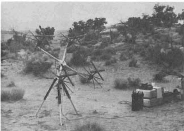
Hammer Ace teams often used a phased array antenna to provide secure satellite communications.
