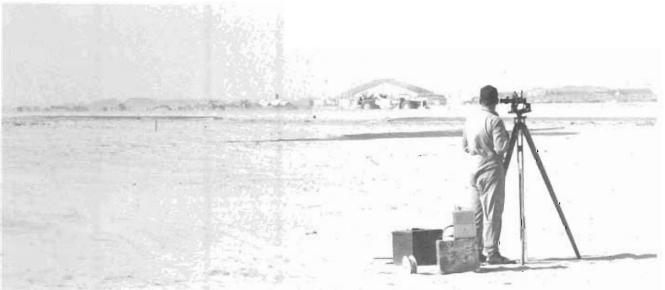
An AFCS sergeant measures the approach angle of an incoming aircraft during a check of the tactical air navigation unit at Chu Lai Marine Air Station, Vietnam.
