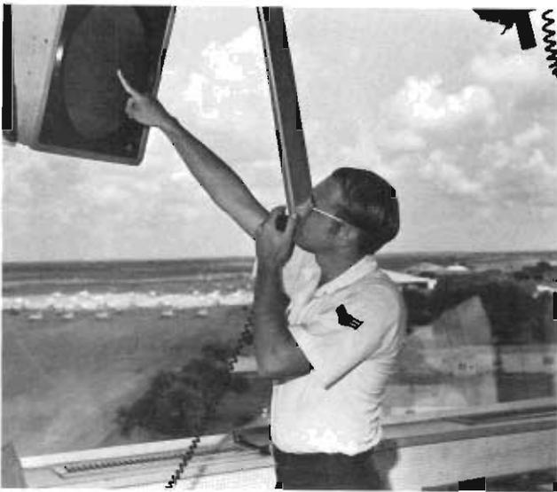
This BRITE II radar facility was added to many AFCC control towers to improve air traffic control services.
