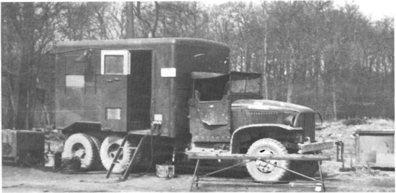
An AACs mobile, low frequency transmitter was used during the Berlin Airlift as a homing beacon.
