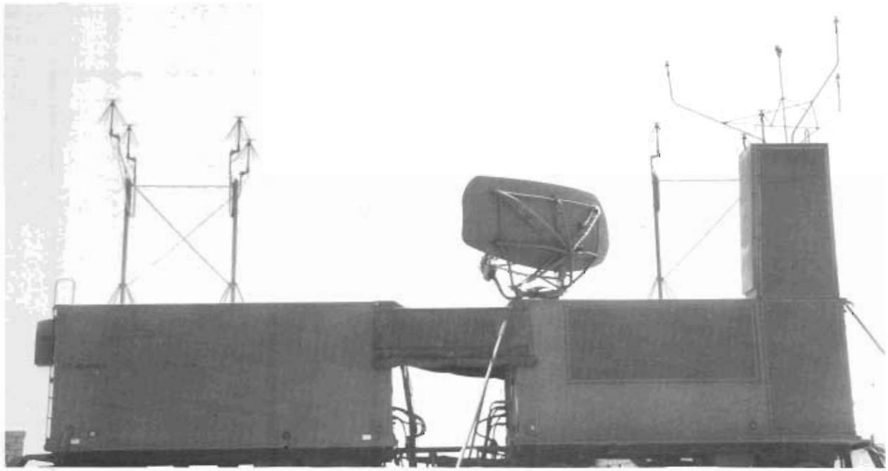
This mobile radar approach control unit provides essential navigational aid to aircraft.
