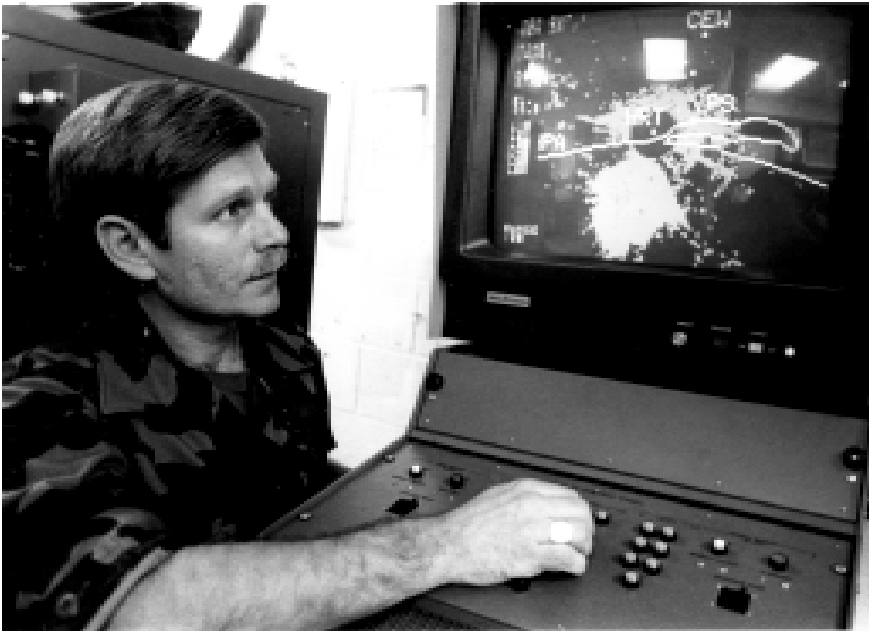
Solid-state electronic weather equipment allows weather forecasters to calculate the intensity and precise location of a storm.
