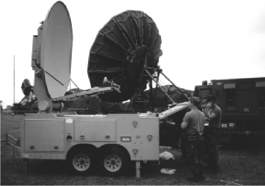
5th Combat Communications Group personnel deploy a lightweight, multi-band satellite communications unit.
