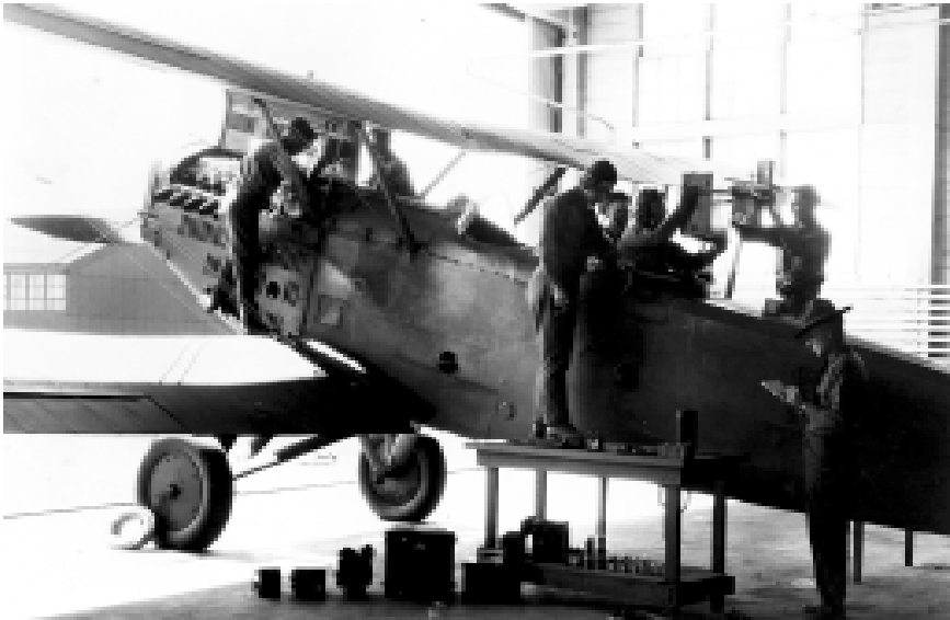
Installing radio equipment, ignition shielding, bonding, and metalizing on a Douglas O-2 at Chanute Field, Illinois, June 1925.
