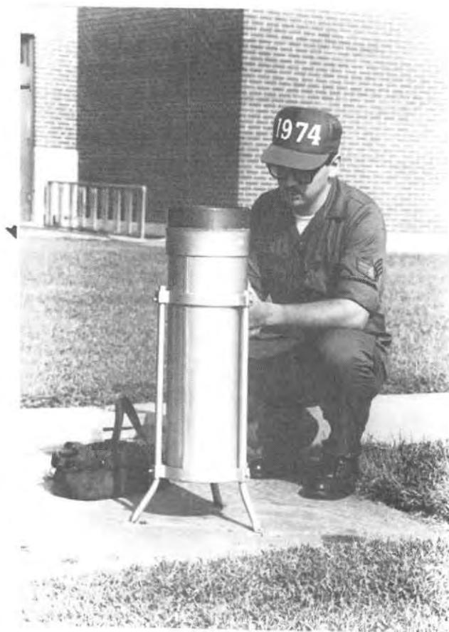
In spite of modern technology, this solid brass ML-17 rain gauge, one of the oldest Air Force weather instruments which originally belonged to the U.S. Army Air Corps, is not scheduled for replacement. SrA. Raymond C. Corethers, a 1974th Communications Group weather equipment technician, is shown adjusting the instrument.
