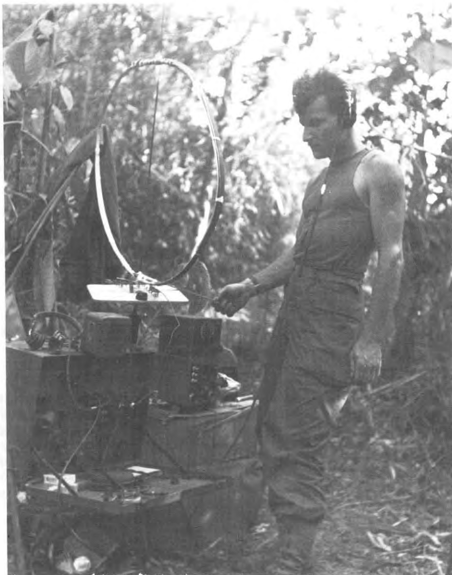
A radio direction finder made of cannibalized parts improvised in the Burma Jungle, 1944.
