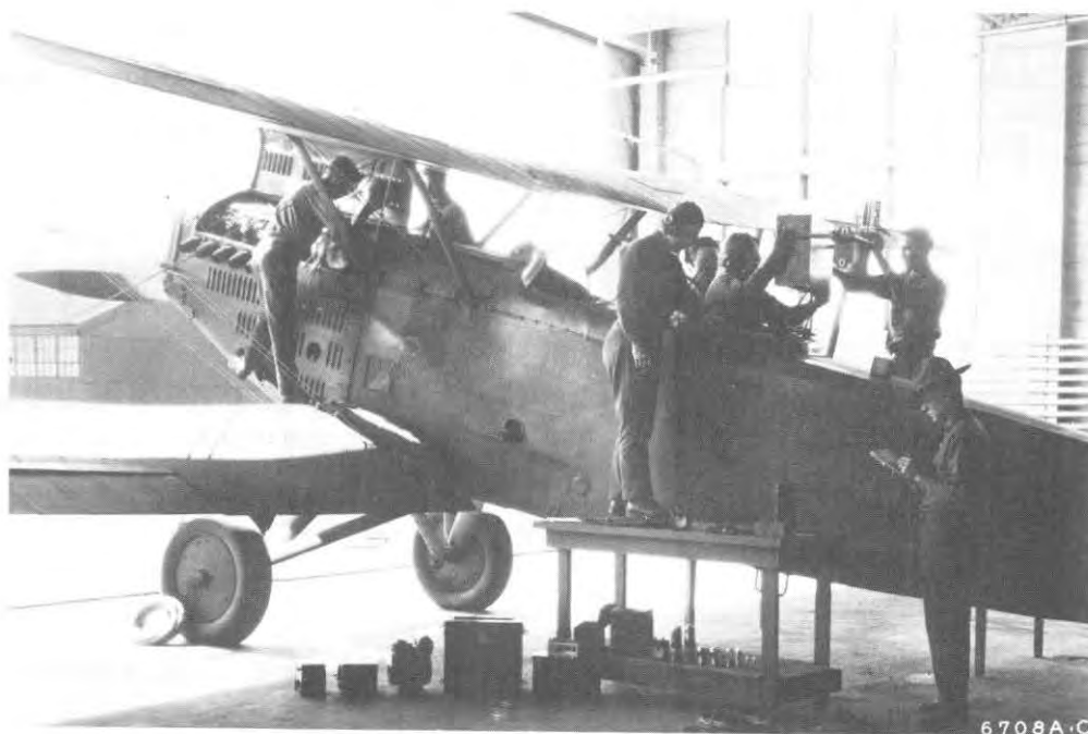
Installation of radio equipment, shield ignition system, bonding and metallizing on Douglas O-2 airplane at Chanute Field, Illinois.
