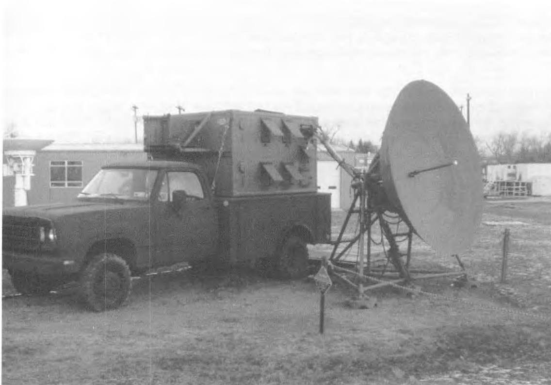
The Electronic Systems Division turned over the first two AN/TSC-94 super high frequency satellite communications ground terminals to the Air Force Communications Service on 17 August 1979.
