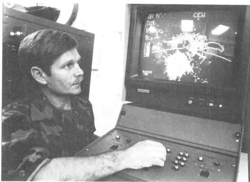
The FPQ-21 can detect precipitation as small as one-hundredth of an inch per hour. This solid-state electronic equipment will allow weather forecasters to calculate the intensity and precise location of a storm, detect how severe the storm will be and how long it will last.
