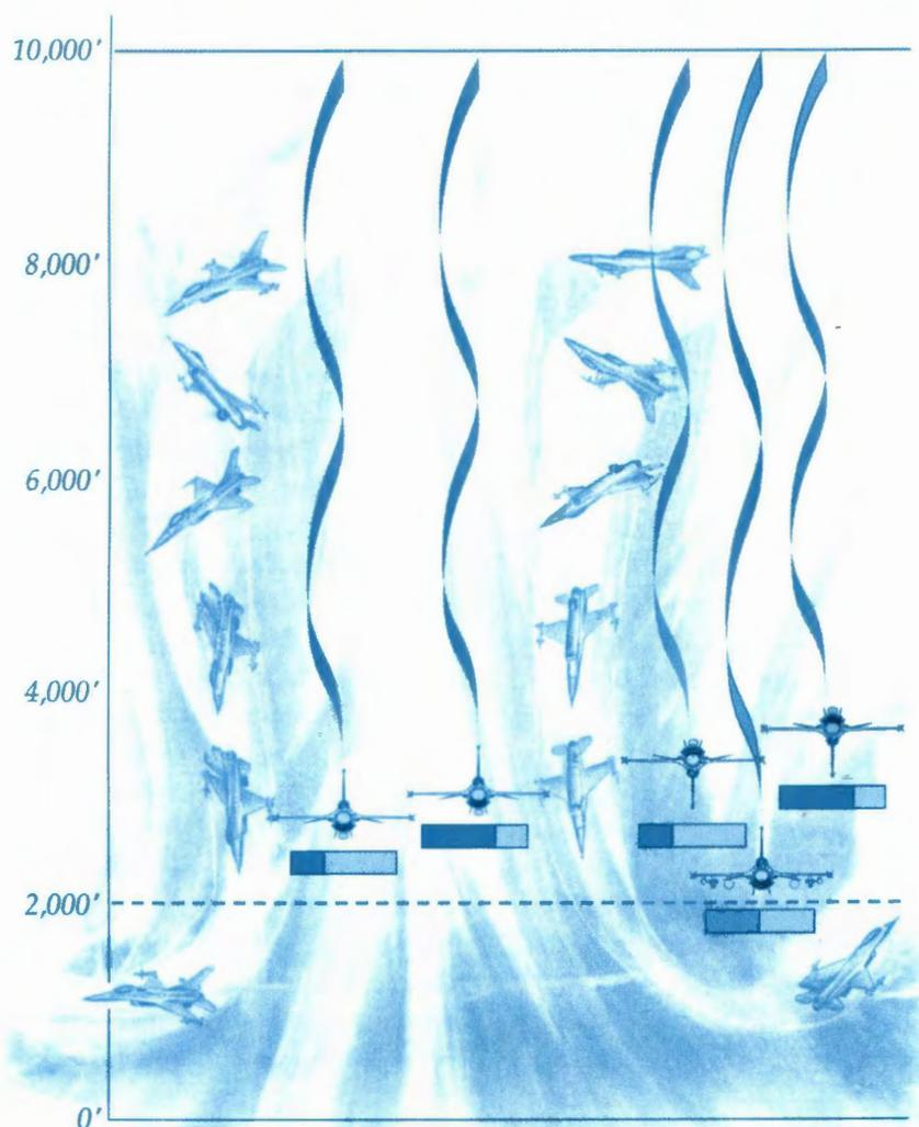
*Cat I recoveries, from both upright and inverted initial conditions, tend to be higher from deep stall initial conditions because the airspeed at the start of the recovery phase was higher and the dive angle was shallower.*
